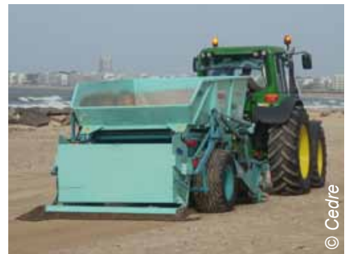
Large beach-cleaning machine powered by a tractor
