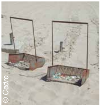
Small baskets made of meshing used to recover solid debris
