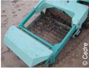
Small, self-propelled beach-cleaning machine
