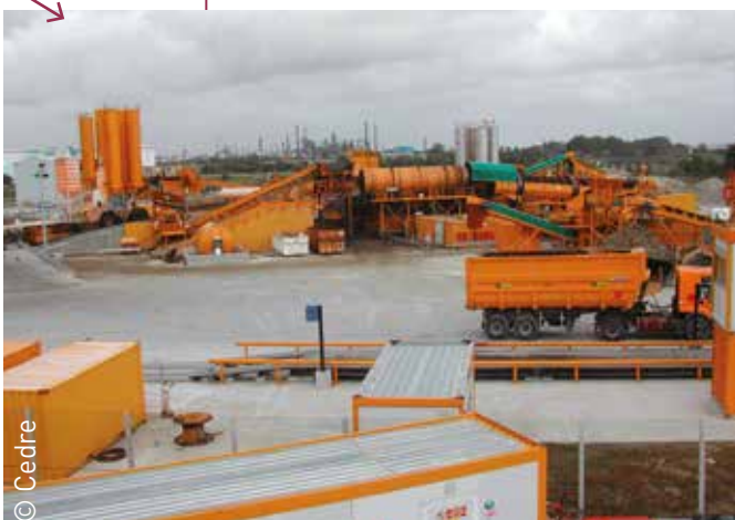
Treatment plant built for sediment washing during the Erika oil spill
